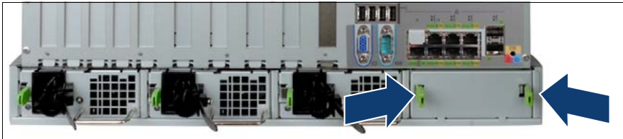
Figure 11: Removing a dummy module from a PSU bay
